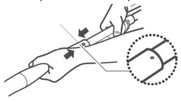
2. Attach lower pole to mop head by aligning the clasp and inserting until pole locks in place
